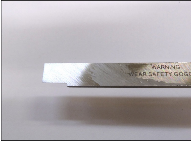
Figure 3. Top View of Chisel Regrind
